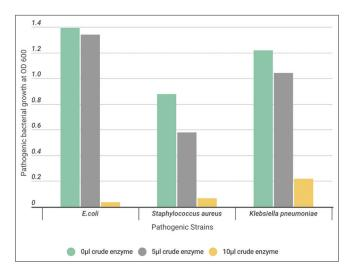
**Figure 9:** The effect of different volumes (0, 5, and 10  $\mu$ l) of crude protease enzyme extracted from *Bacillus subtilis* on the pathogenic strains.
